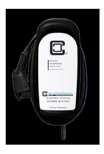
The HCS-40 is a cost-effective Level 2 charger that operates on 208 three-phase or 240 single-phase Vac and delivers up to 7.7 kW while charging. The 25-ft cord provides ample reach for convenient charging. The unit is designed to take the wear and tear of everyday use. The NEMA-4 watertight, rugged enclosure provides safe outdoor installation and protection. It can be wall or pedestal mounted.
