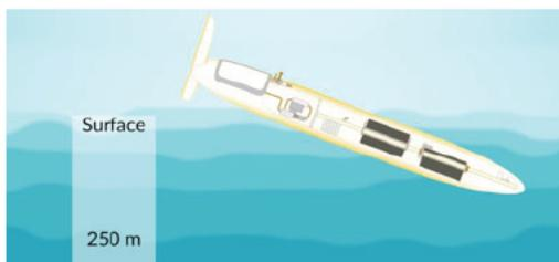
This 2020 Telly Award-winning video highlights the research by the NOAA Pacific Marine Environmental Lab into currents in the Solomon Sea using an autonomous Ocean Glider to collect data about current speed and direction as well as water temperature. The resulting data is used to enhance El Niño weather event long range forecasting.
