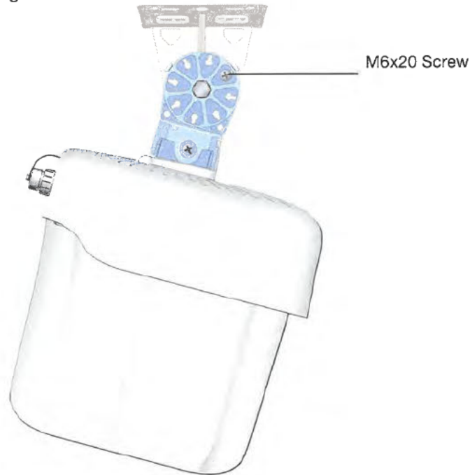
Figure 6 Adjusting the Inclination of the AP
