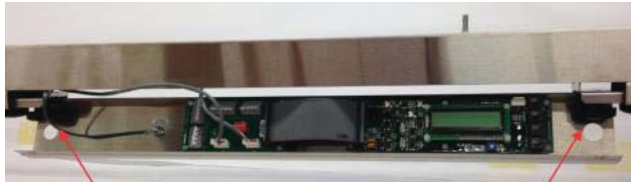
Use Thumbscrew to hold control module
