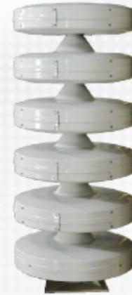
Federal Signal's Modulator II Siren offers the same proven technology as the original Modulator with the exception of a smaller compact chassis. Modulator II provides a flat frequency response up to 2000Hz producing intense warning signals and digital voice messaging over a large area. The Modulator II design enables the siren to produce a high sound level and intelligible voice communications.
