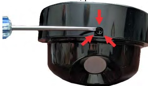
Figure 3: TUS-300 Locking Tab Movement
