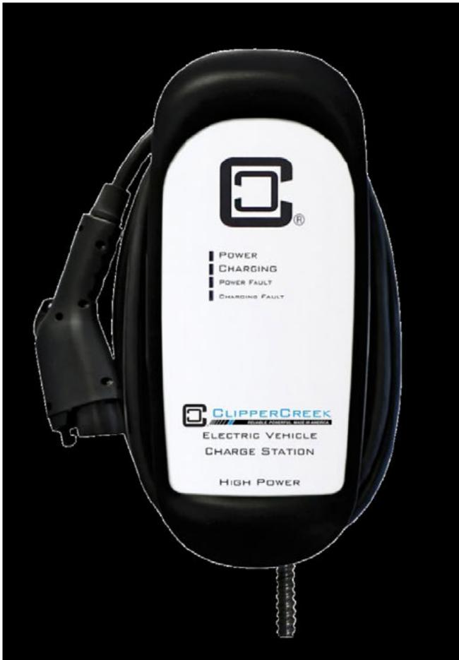
The HCS-40 is a cost-effective Level 2 charger that operates on 208 three-phase or 240 single-phase Vac and delivers up to 7.7 kW while charging. The 25-ft cord provides ample reach for convenient charging. The unit is designed to take the wear and tear of everyday use. The NEMA-4 watertight, rugged enclosure provides safe outdoor installation and protection. It can be wall or pedestal mounted.
